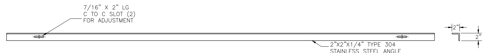
TYPICAL HORIZONTAL SUPPORT ANGLE SCALE: NONE
