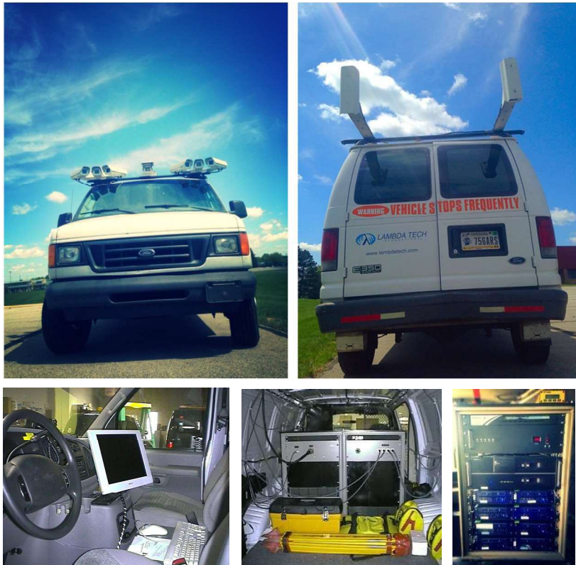
GPSVision Data Collection Vehicle to be used for the right of way survey proposed project.
