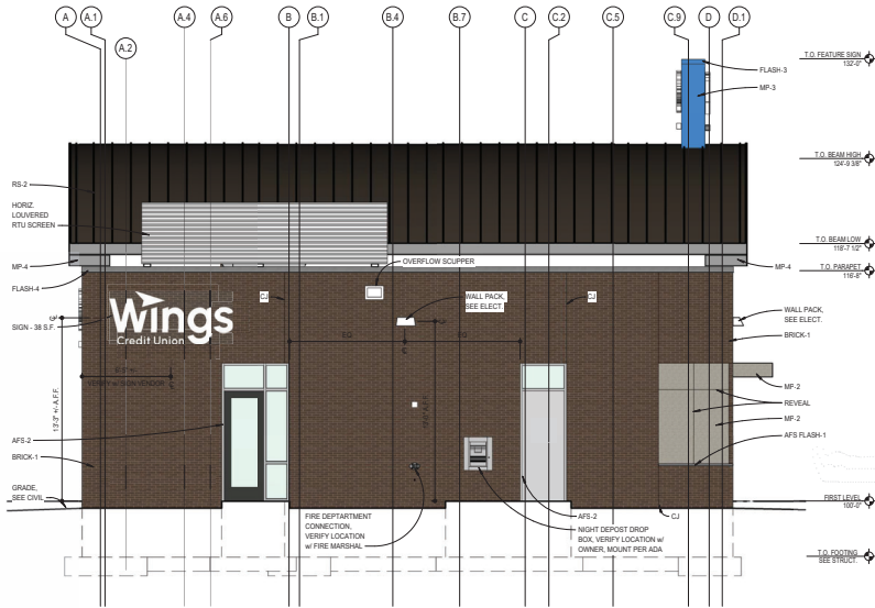
SOUTH BUILDING ELEVATION 1/4" = 1'-0"
