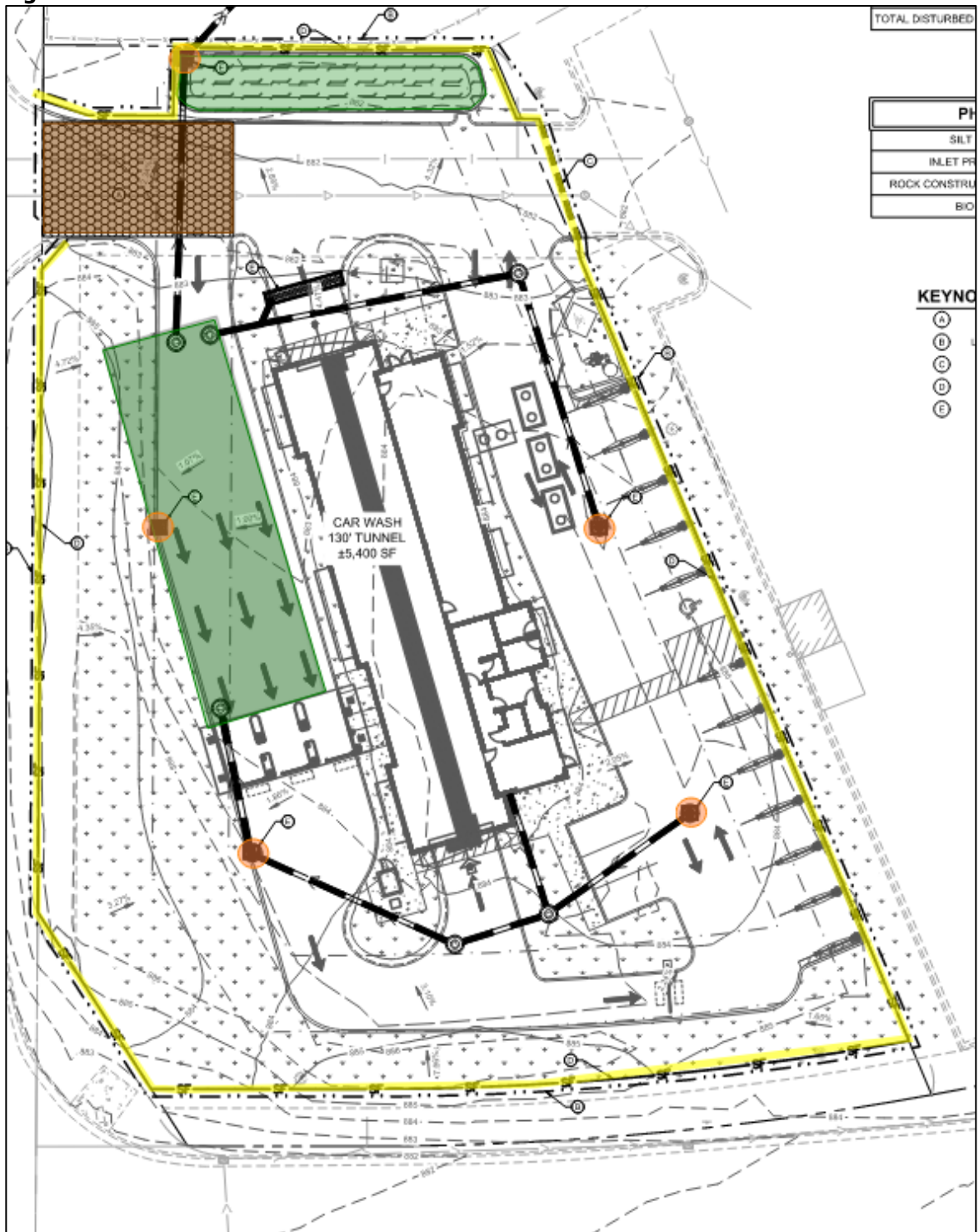
Figure 2. Erosion and Sediment Control Plan
